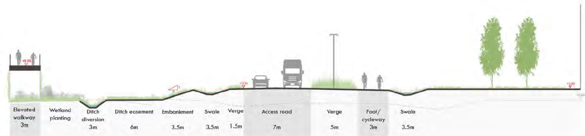
Figure 5.12: Illustrative section through main access road
